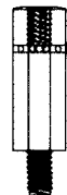
FRONT VIEW 18-8 SS MALE FEMALE THREADED HEX STANDOFF 3/16 HEX 1/2 LENGTH 2.56 SCREW SIZE 8 REQUIRED
